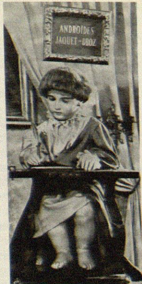
1 The Jaquet-Droz Writer (circa 1774). The little boy is 28 inches tall, carved from wood, and composed of a very complicated mechanism which still works. It has carefully written, "I do not think, therefore I will never be." (Photograph courtesy of Editions du Griffon, automaton in Neuchâtel Museum)
